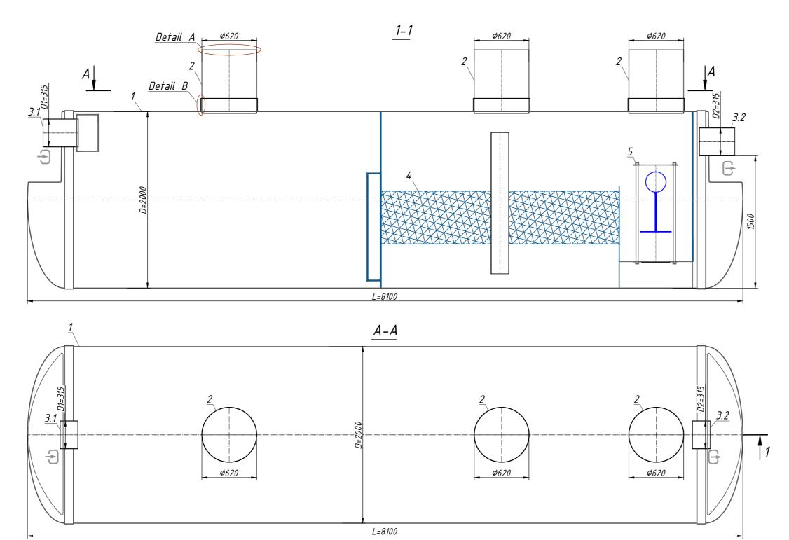
\*H-depth of the inlet connection, mm (in standard equipment H up to 2000 mm). H take a multiple of 50mm. When filling the manhole A.1-the overal height of the product is less than 200mm; A.2-the total height of the product is bigger
